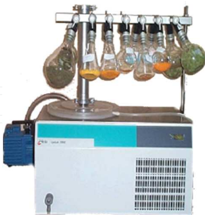
Fig. 3. Freeze-dryer with several Erlenmeyer flasks connected containing different frozen solutions.
