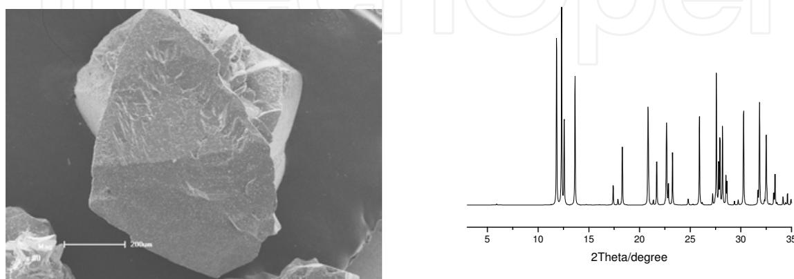
Fig. 10. SEM image and XRD pattern of CoZnPO<sub>4</sub>-VII.
