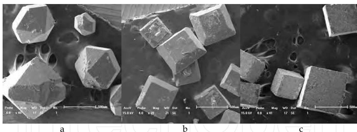
Fig. 5. SEM images of the large crystals of three cobalt-zinc phosphates : (a) crystal of CoZnPO<sub>4</sub>-I with elongated hexagonal-dipyramid morphology;(b) CoZnPO<sub>4</sub>-II crystal with square bipyramid morphology; (c) CoZnPO<sub>4</sub>-III crystal with cubical-like morphology.
