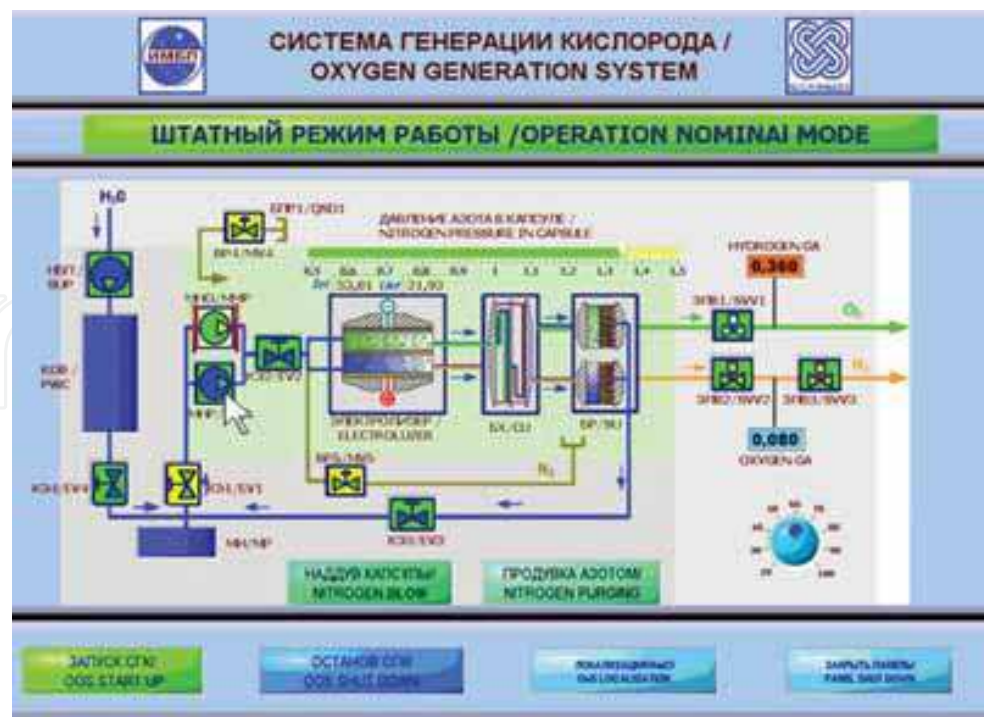
Fig. 11. Front panel of the ‘OGS’ virtual simulator subroutine in ‘ OPERATION NOMINAL MODE ’ (НБП/SUP=supply unit pump; KOB/PWC=pre-purification water container; КЭИ/EVI=electromagnetic valve; МНП/RMP and МНП/RMP=main micro-pump and reserve micro-pump; БХ/CU=cooling unit; БП/SU=separator unit; GA=gas analyzer).
