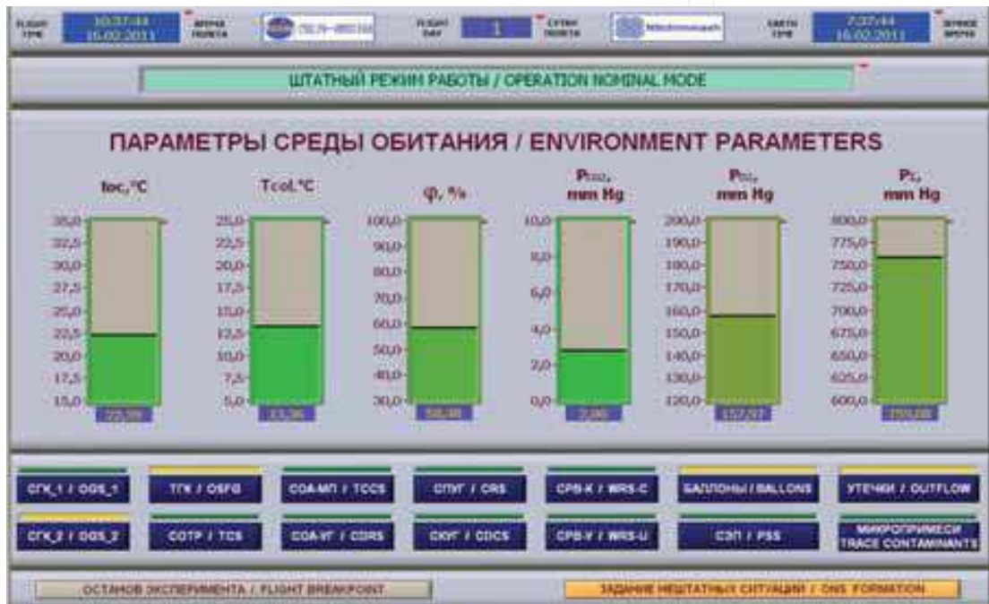
Fig. 7. Control panel of the 'PMM atmosphere' simulation model, where: t_{oc} , °C, T_{col} , °C, \varphi , %, p_{CO_2} , mm of Hg, p_{O_2} , mm of Hg, p_{\Sigma} , mm of Hg = controllable parameter values.
