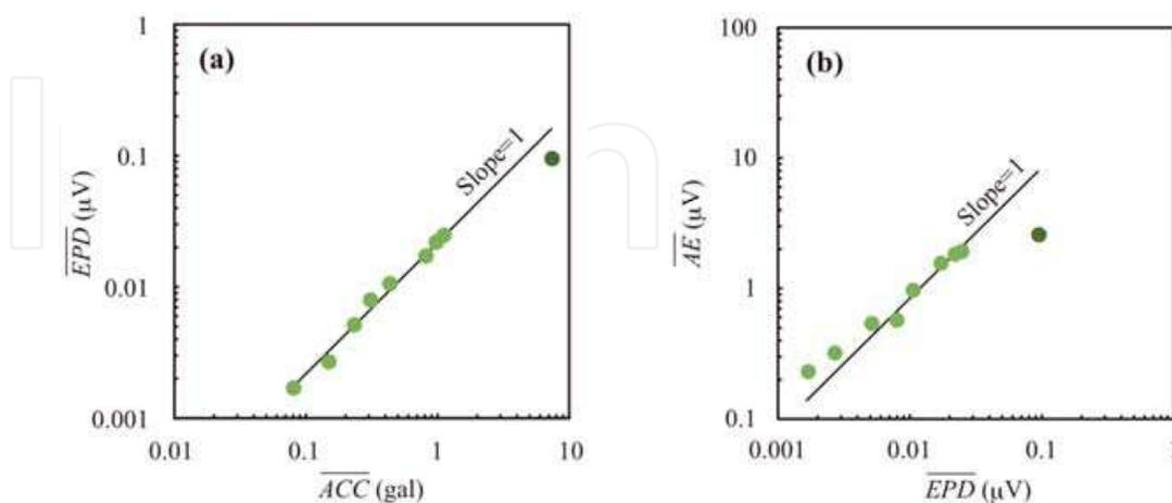
Fig. 15. (a) Positive relation between the average of the earth potential difference ( $\overline{EPD}$ ) and the average of the ground up-down acceleration ( $\overline{ACC}$ ). (b) Positive relation between the average of the atmospheric electricity ( $\overline{AE}$ ) and  $\overline{EPD}$ . Linear lines with the slope of 1 are obtained from the plots, excluding the dark plots. Modified from Okubo et al. (2007)
