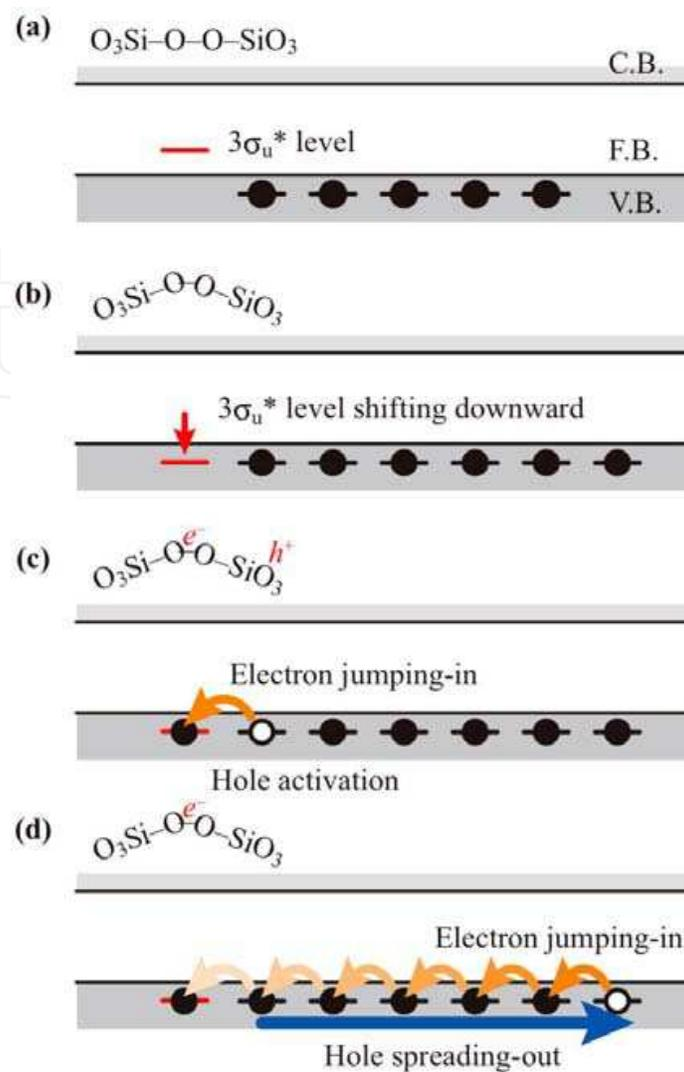
Fig. 7. Band model of stress-activation of a positive hole in the case of quartz. (a) Normal state. (b) Downward shift of the unoccupied  $3\sigma_u^*$  level accompanying structure deformation around a peroxy bond under subjection of a load. (c) Jump-in of an electron and activation of a positive hole. (d) Movement of a positive hole through the valence band by successive electron-hopping steps. Modified from Takeuchi et al. (2010)
