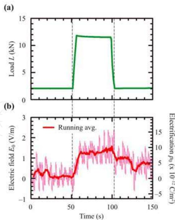
Fig. 5. Typical example of experimental measurements. (a) Loading profile  $L$ . (b) Electric field  $E_0$  at the rock top surface and surface charge density calculated as  $p_0$ .  $E_0$  and  $p_0$  denote differences from the values at the initial load  $L = 2$  kN. Modified from Takeuchi et al. (2010)
