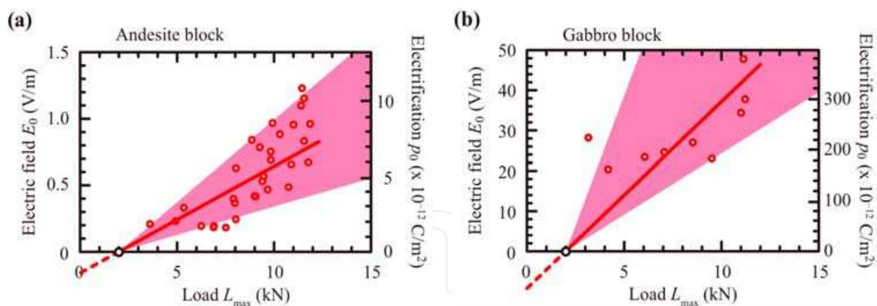
Fig. 6. Electric field  $E_0$  and electrification  $p_0$  measured on the top surface of the upper unstressed volume of the rock block shown against the maximum load  $L_{\max}$  applied to the lower volume of the rock. (a) Quartz-bearing andesite. (b) Quartz-free gabbro.  $E_0$  and  $p_0$  denote differences from the values at the initial load  $L = 2$  kN. Modified from Takeuchi et al. (2010)
