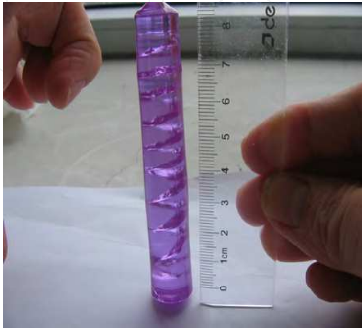
Fig. 2.1 The cracking \text{Nd}^{3+}:\text{NaY}(\text{WO}_4)_2 crystal.
