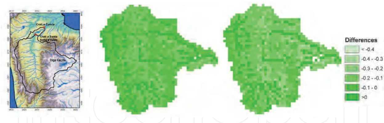
Fig. 15. Location of the Crati River Basin (left) and spatially distributed percentage changes in annual actual evapotranspiration (middle) and in actual evapotranspiration during the April–September irrigation period (right) simulated using RegCM (2070-2099 vs 1961-1990) (adapted from Senatore et al., 2011).
