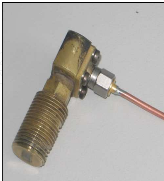
Fig. 20. The antenna for the PIT microwave sensor
