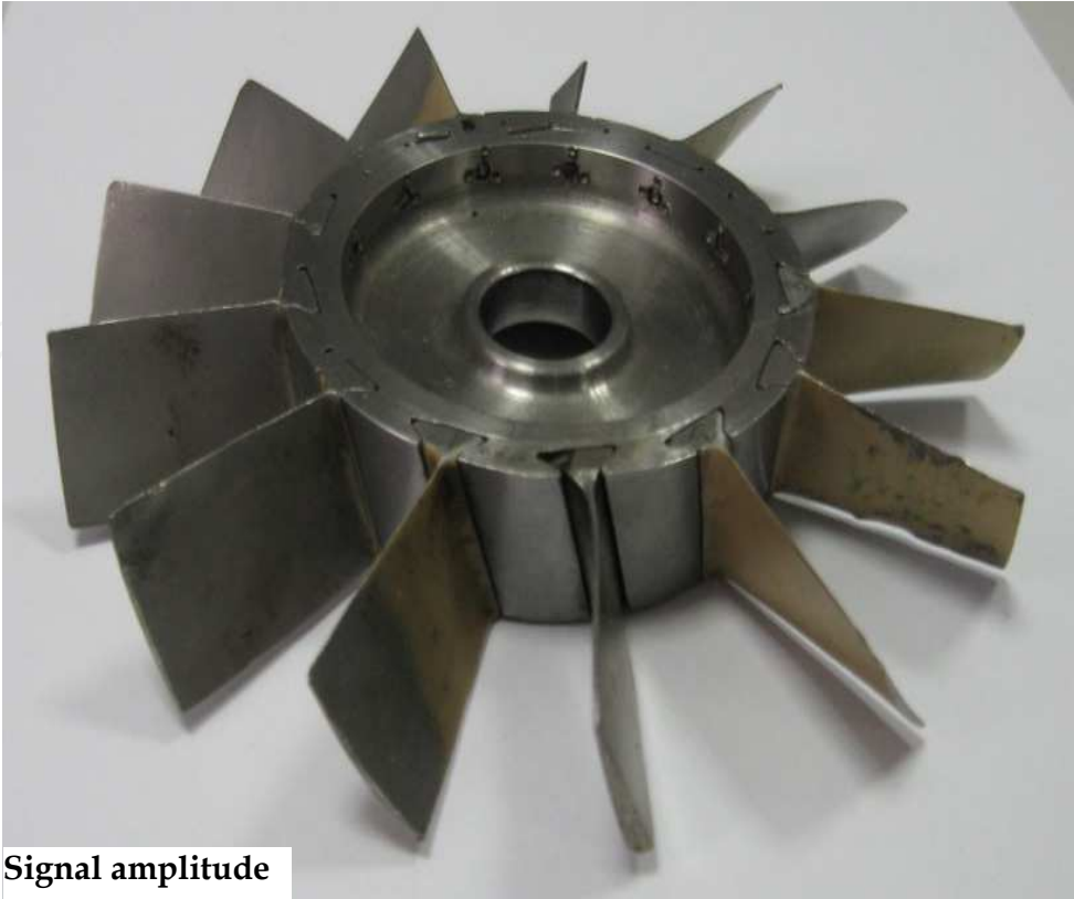
Fig. 8. View of the turbine disc with blades
