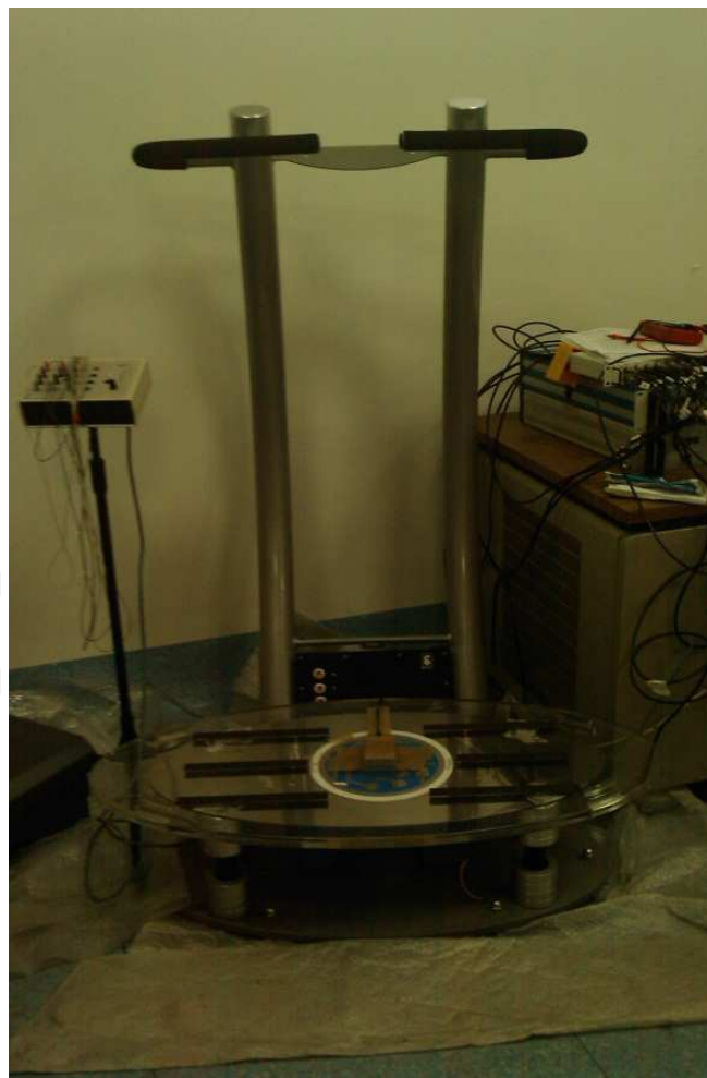
Fig. 4. Vibrating platform used to deliver vibratory stimulation (see text).
