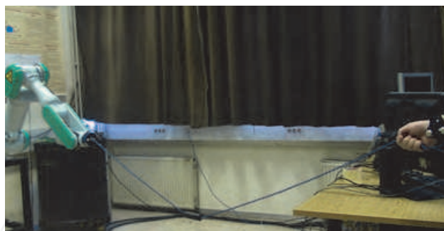
Fig. 14. Experimental setup for cooperative human-robot rope turning.
