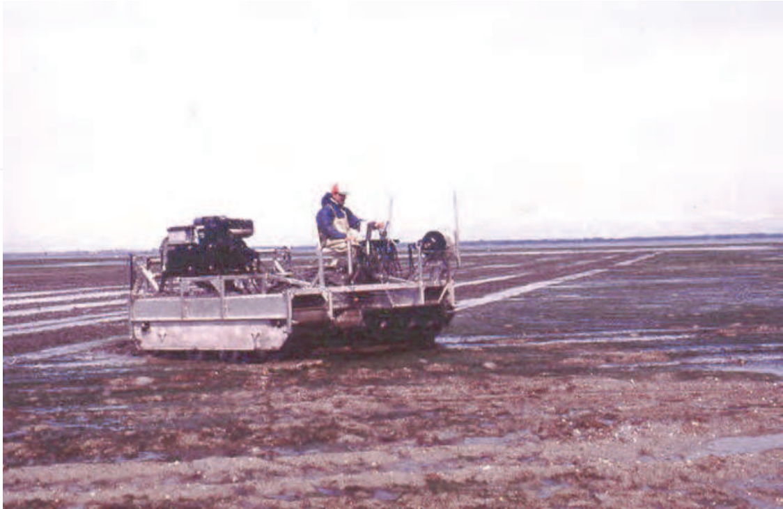
Fig. 5. Seeder machine combined to remove oyster shells
