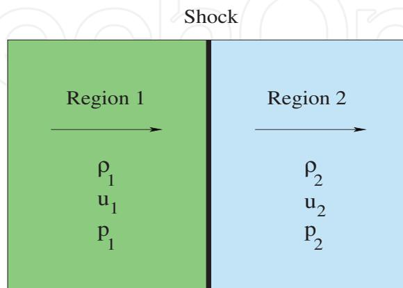
Fig. 7. A schematic diagram of a shock wave situation with the indicated density, velocity, and pressure for each region.
