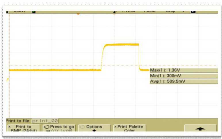
Fig. 13. Voltage across PV panel
