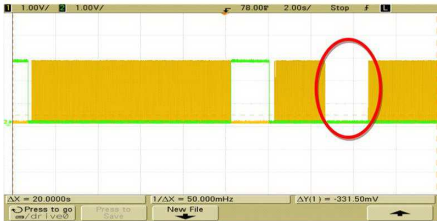
Fig. 16. No switching at Gate of NMOS3 when V_{ref} is less than V_{pv}
