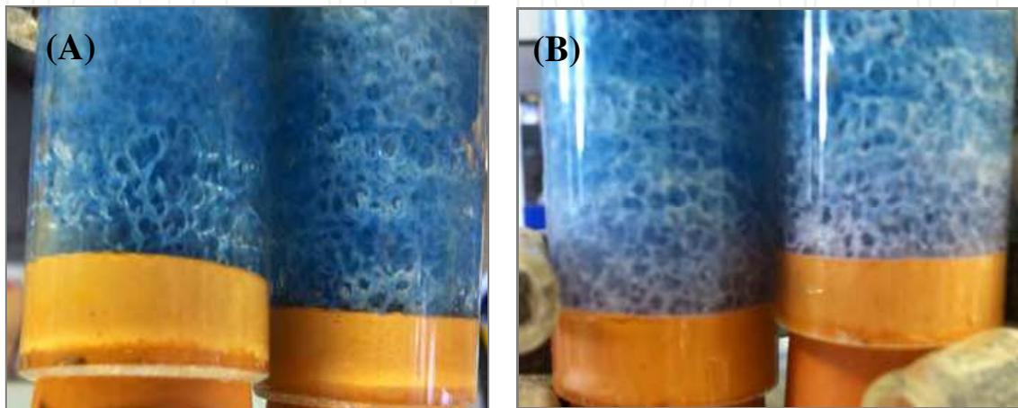
Fig. 10. Reactors containing *Serratia* sp. biofilm on polyurethane foam (A) before and (B) after treatment with  $\text{N}_3\text{NdO}_9 \cdot 6\text{H}_2\text{O}$  (54.5 hours); a purple colour can be seen at the bottom of the reactors, in B.
