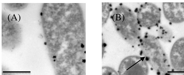
Fig. 3. TEM micrographs of pre-palladised *E. coli* cells before and after the recovery of PGMs from a model solution. The initial Pd loading was set to 5 wt% (A) and increased to 20 wt% (total metal loading) following exposure to the Pt/Pd mixture (B). Scale bars are 500 nm.
