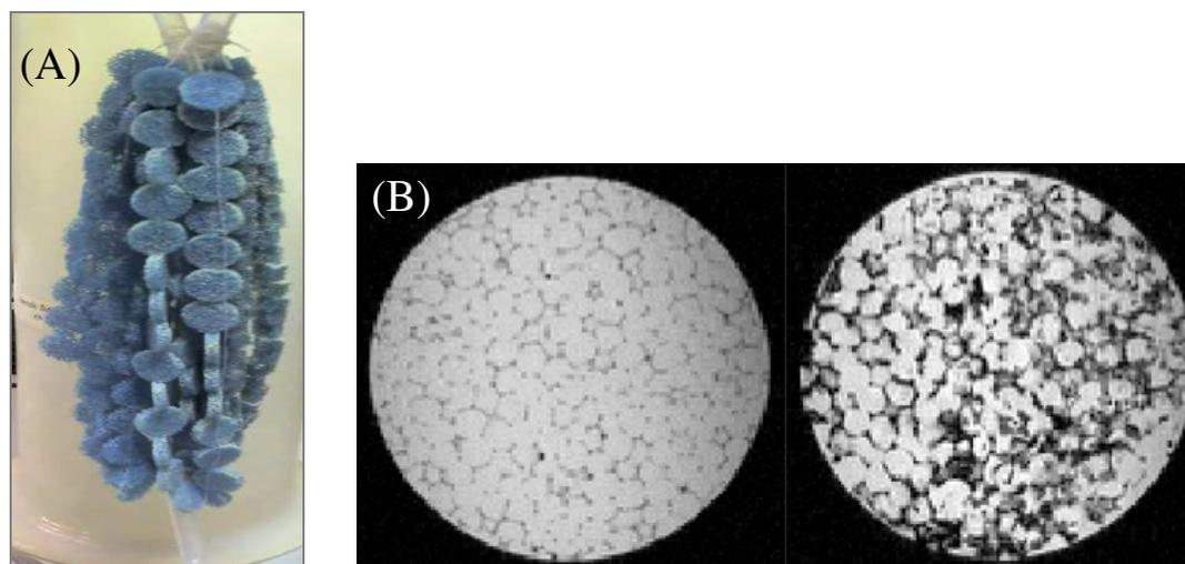
Fig. 8. (A) *Serratia* sp. biofilm grown on polyurethane reticulated foam discs. (B) Magnetic resonance imaging of discs with or without *Serratia* biofilm. MRI image of discs (diameter 20 mm, left) containing polyurethane foam only and *Serratia* sp biofilm coated polyurethane foam (right). The biofilm in a  $T_2$ -weighted spin-echo image is the darker regions, due to a reduced  $T_2$  of water (P. Yong, M.L. Johns and L.E. Macaskie, unpublished).
