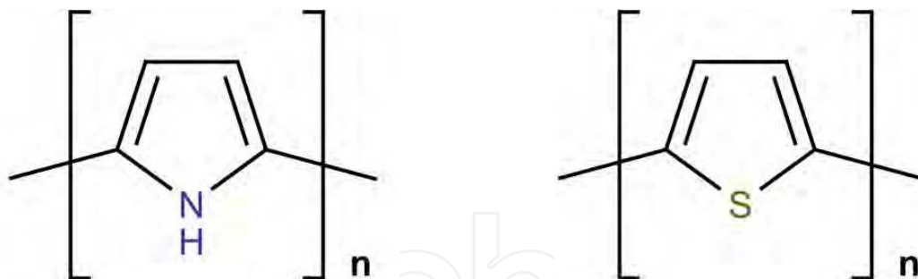
Fig. 12. Chemical structure of Poly(pyrrole) PPy (left), Polythiophene (PTh) (right) [7]
