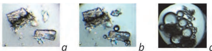
Fig. 14. HSM images for 5 at a) 25 °C; b) 90°C – slow release of crystallization water; c) 160°C – lactamization and melting 84 .
