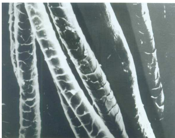
Fig. 1.2. SEM graph of untreated wool.
