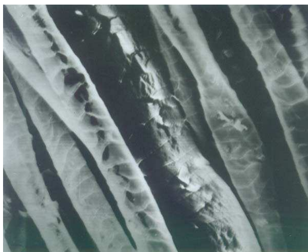
Fig. 1.3. SEM graph of sulphamic acid-treated wool.
