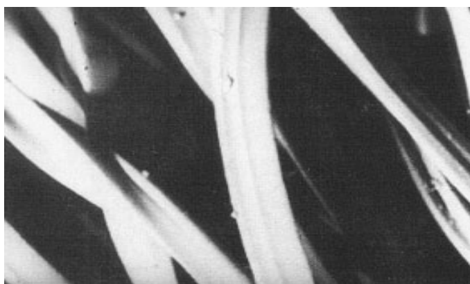
Fig. 2.2. SEM of treated polyester fabric with ethoxide (16) .
