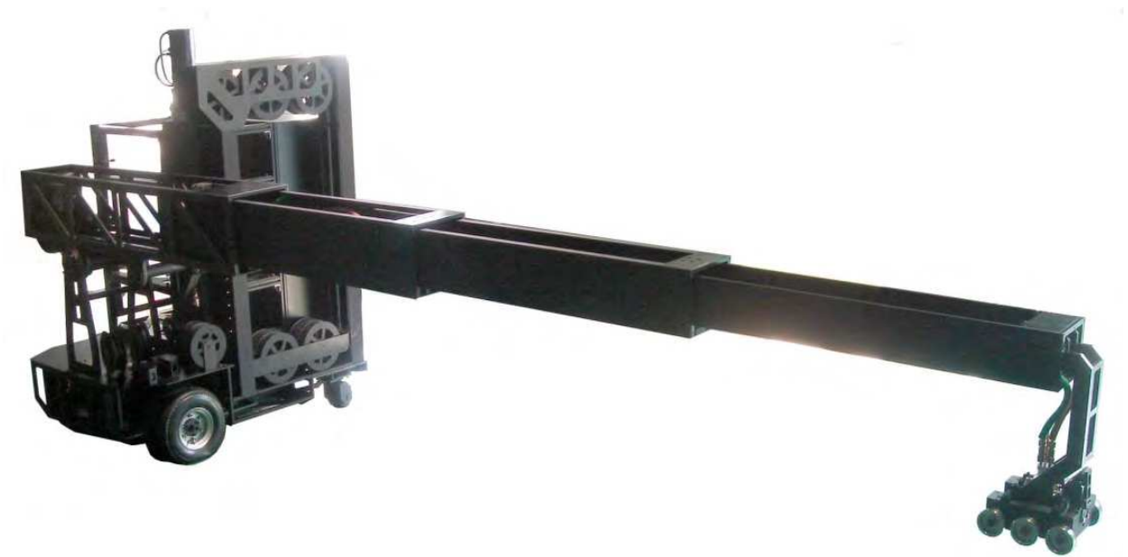
Fig. 2. APSCR stretches its arm up to 3.8 m.
