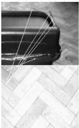
Fig. 17. False matching generated by SIFT matching.
