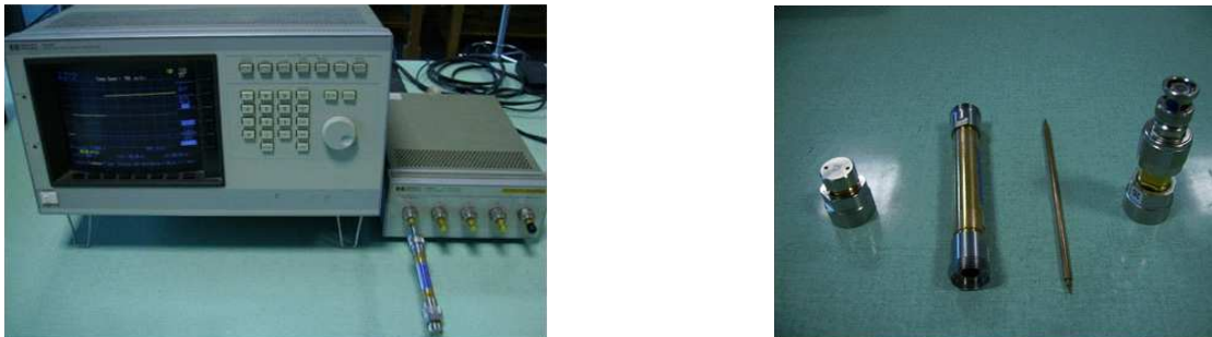
Fig. 15. The frontal panel of the HP 54120B digitalizing oscilloscope with rise time t_r = 10 ps (left). The coaxial probe (Maury Microwave Airline, model no. 2653S10, length \ell = 10.5 cm used in the measurement setup (right).
