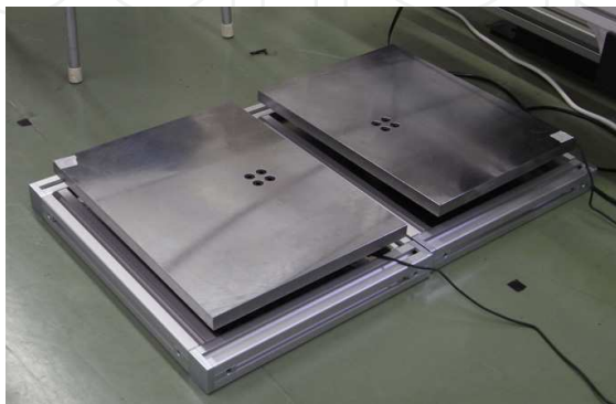
Fig. 5. Force detection plates for measuring feet pressure
