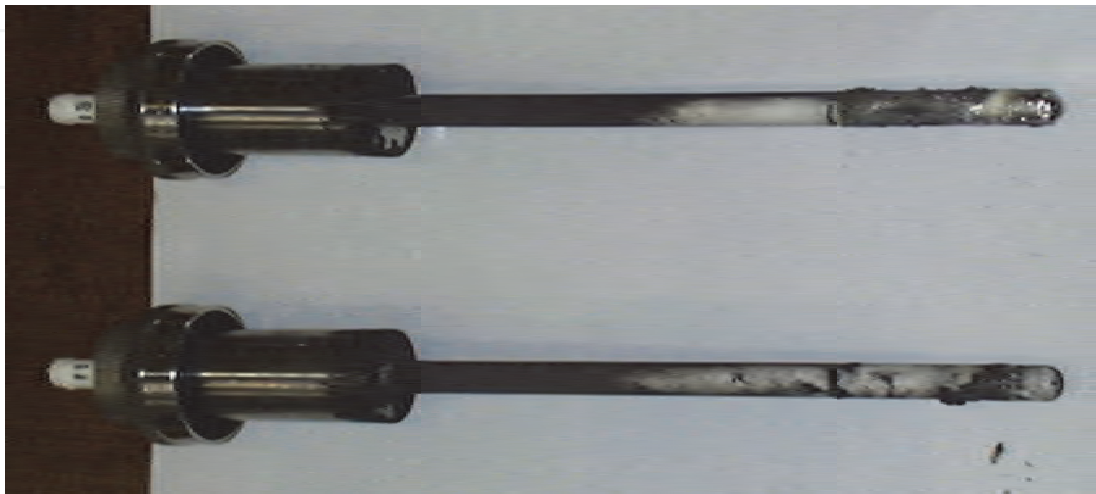
Fig. 11. Appearance of oxygen sensors after measurement in liquid LBE using the comparison apparatus of oxygen sensors.
