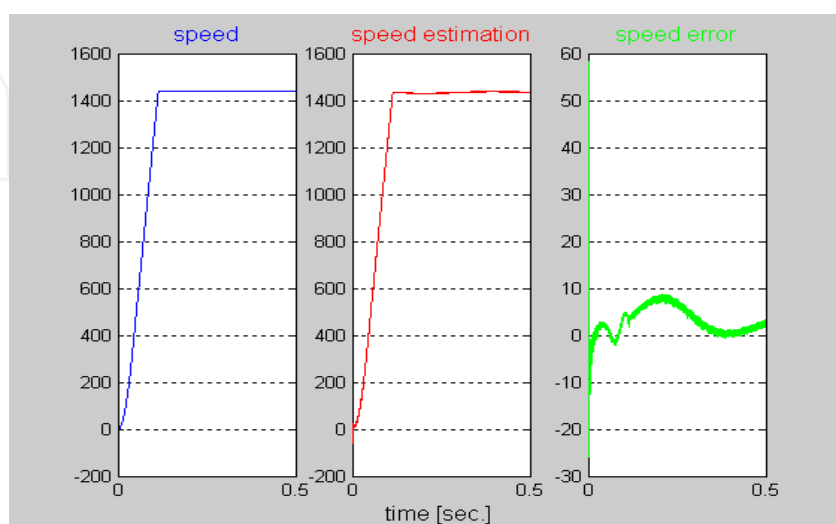
Fig. 22. Speed, estimated speed and speed error for a robust controlled starting process.
