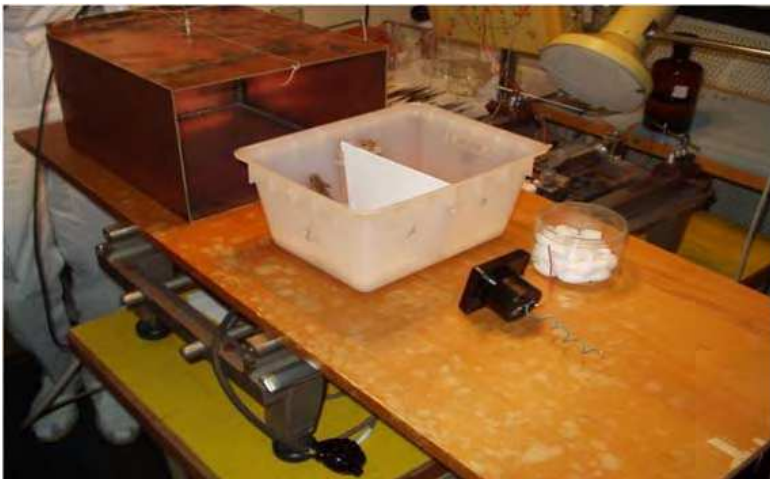
Fig. 26. Exposure system for research of electromagnetic field and biological system interactions
