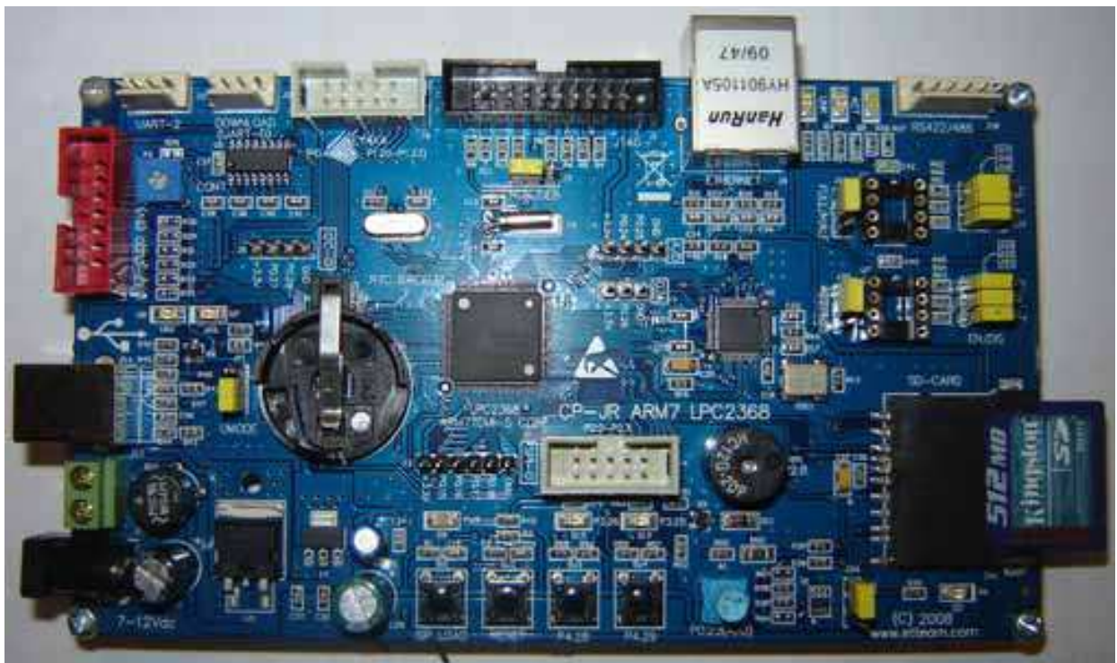
Fig. 5. The development board of LPC2368 microcontroller
