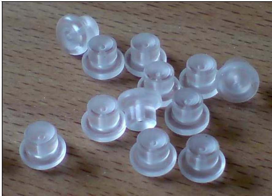
Fig. 2. Poly (2-hydroxyethylmethacrylate) scaffolds – upper parts of hybrid replacements
