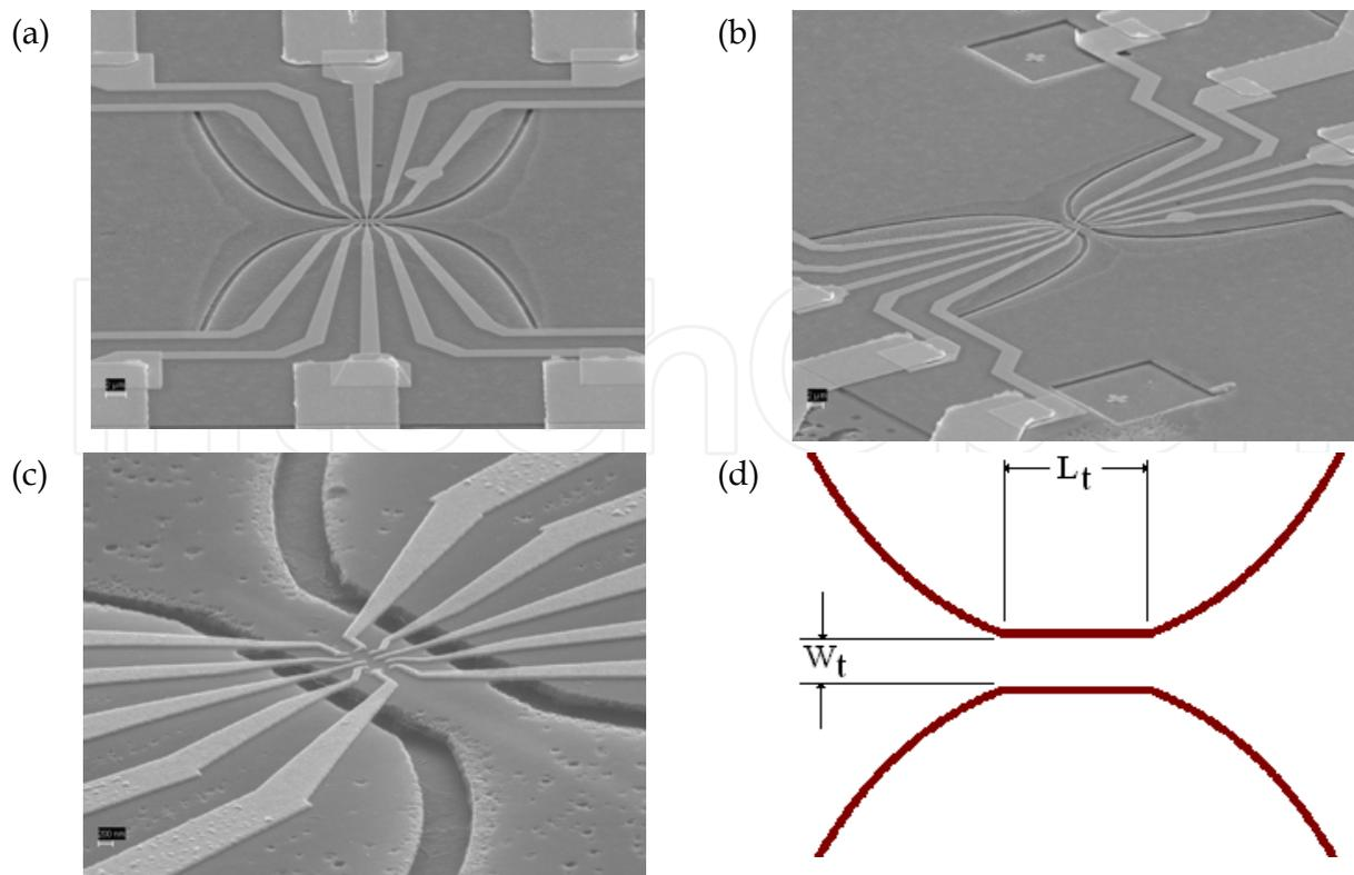
Fig. 2. SEM images of an exponential waveguide with a cutoff frequency of 75 MHz and throat width of  $\sim 1.5 \mu\text{m}$ . The darker region around the waveguide shows that the area is suspended, which was achieved by an HCl etch to remove the sacrificial layer below the 2DEG, (a), (b) and (c). (d) Schematic of waveguide, center region is the throat (pipe waveguide) with width  $W_t$  and length  $L_t$ . The outer curves are the exponential portion of the waveguide
