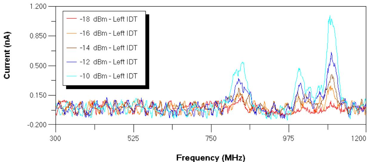
Fig. 8. A frequency sweep of varying RF powers while the center QPC of the sample in Fig. 4 is held at  $-0.8$  V. The first peak is at 840 MHz with a current of 540 pA and a velocity of 3,368 m/s, the second peak at 1.005 GHz with a current of 472 pA and a velocity of 4,020 m/s, the third peak is at 1.095 GHz with a current of 1.098 nA and a velocity of 4,380 m/s
