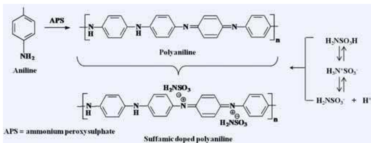
Fig. 15. Proposed mechanism of sulfamic doping into PANI NFs.
