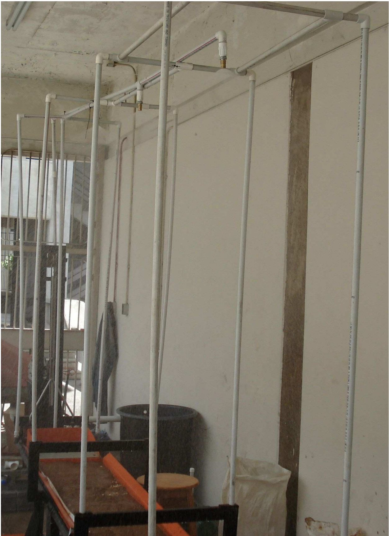
Fig. 2. The rainfall simulator with the soil bed
