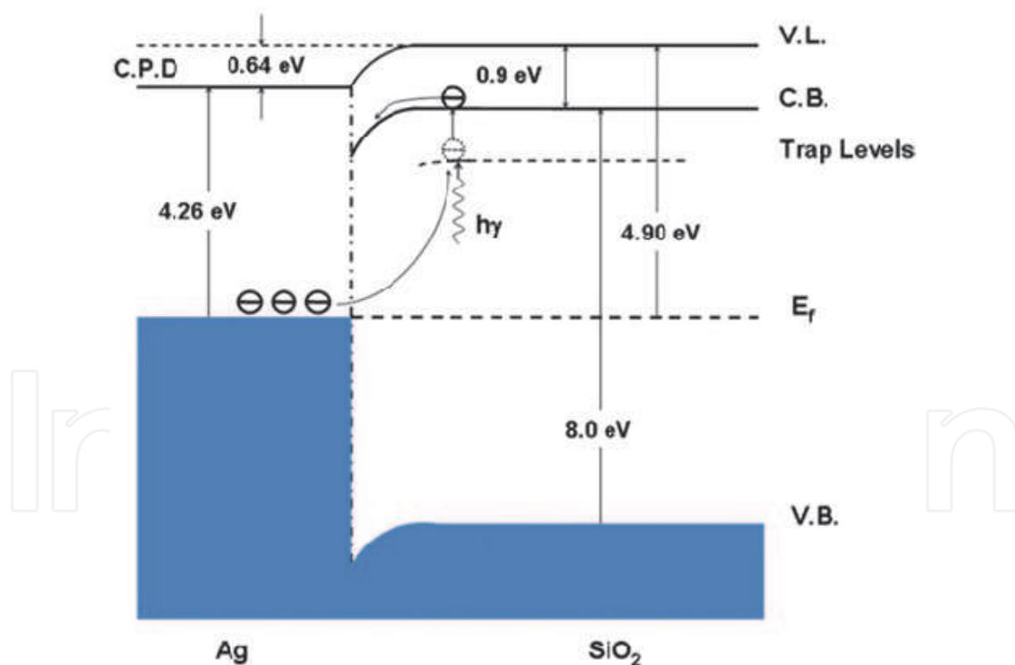
Fig. 12. The schematic band structure of the Ag- $\text{SiO}_2$  contact. C.P.D., V.L., C.B., V.B. and  $E_f$  denoted the contact potential difference, vacuum level, conduction band, valence band and Fermi level, respectively. [14]
