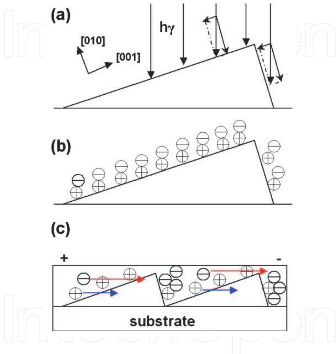
Fig. 20. (Color online) (a) The schematic drawing under the irradiation. (b) The difference of the carry destiny caused by the miscut angle. (c) The transient movement of the photogenerated carriers of the  $\text{La}_{0.6}\text{Ca}_{0.4}\text{MnO}_3$ . [15]
