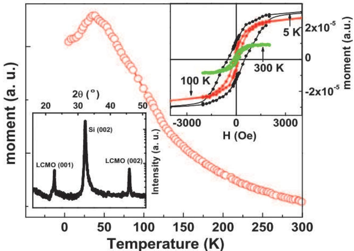
Fig. 21. The magnetic moment as a function of temperature of the junction. The left and right insets show the XRD pattern and magnetic hysteresis loop, respectively. [16]
