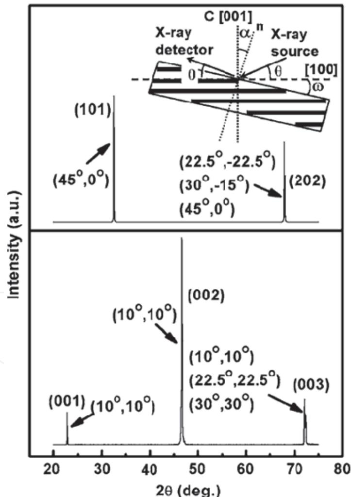
Fig. 1. X-ray diffraction patterns of tilted STO crystals. The inset shows the configuration of  $\theta$ - $2\theta$  scan. To get different diffraction peaks, (00 $l$ ), (10 $l$ ) and (20 $l$ ),  $\omega$  was adjusted as shown in the angle arrays ( $\alpha$ , $\omega$ ) for different  $\alpha$ . [11]
