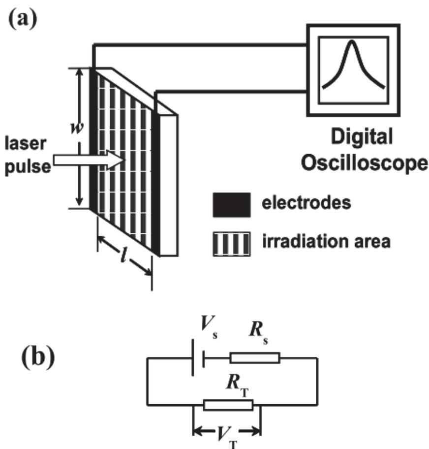
Fig. 5. (a) Schematic of the optical response measurement setup.  $l$  and  $w$  denote the length and width of the irradiated area, respectively. (b) Corresponding equivalent electrical scheme of the single crystal along the  $l$  direction. [12]
