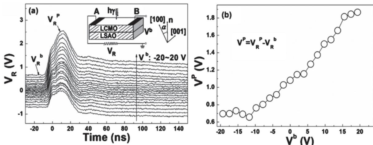
Fig. 17. (a) The photovoltaic pulses for  $\text{La}_{0.6}\text{Ca}_{0.4}\text{MnO}_3/\text{LSAO}$  under the illumination of a 248 nm laser at different biases recorded by an oscilloscope with an input impedance of 50. The inset displays the schematic circuit of the measurement. (b) The photoinduced voltage  $V^P$  defined by  $V^P = V_R^P - V_R^b$  as a function of the applied bias  $V^b$ . The inset shows that  $V_R^P$  as a function of the applied bias  $V^b$ . [15]
