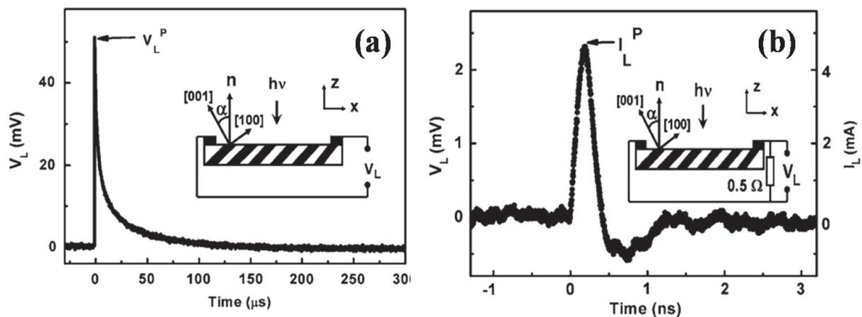
Fig. 2. (a) A typical open-circuit photovoltage and (b) a typical photoresponse signal with a  $0.5 \Omega$  resistance in parallel with the STO single crystal under an excitation of 25 ps duration and 355 nm laser pulses. The tilted degree  $\alpha$  is  $15^\circ$ . The inset displays the schematic circuit of the measurement.  $V_L^P$  and  $I_L^P$  denote the peak value of the transient photovoltage and transient photocurrent, respectively. [11]
