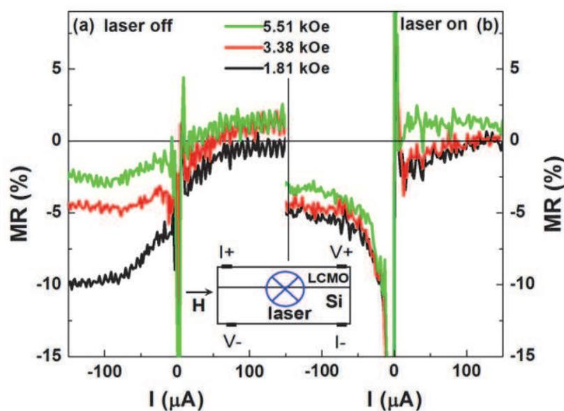
Fig. 26. The dependence of MR values of the junction on bias current in 1.81, 3.38 and 5.51 kOe fields at room temperature. The  $H$  was parallel to the junction interface and perpendicular to the direction of light which was parallel to the junction interface. [16]
