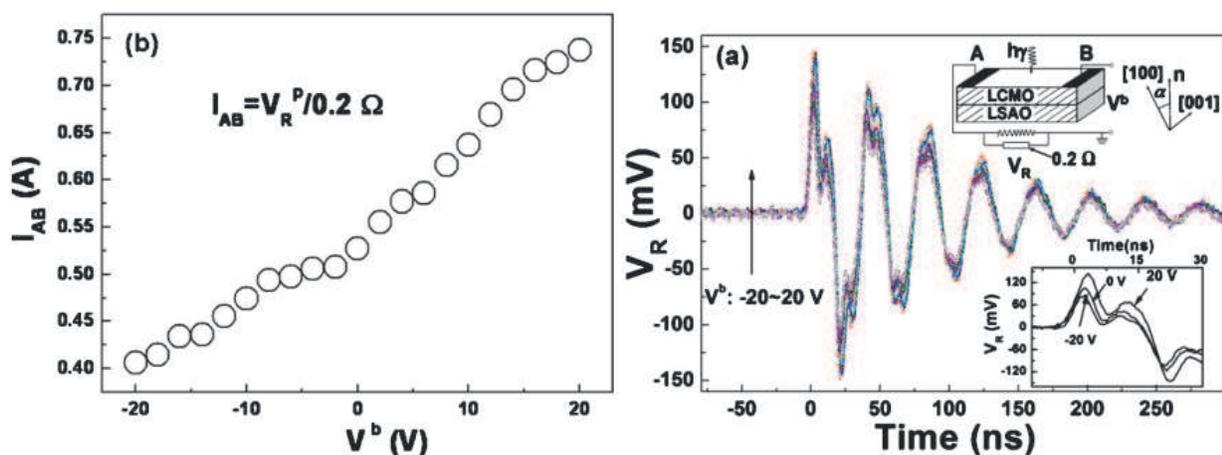
Fig. 18. (Color online) (a) The photovoltaic pulses and (b) peak photocurrent for  $\text{La}_{0.6}\text{Ca}_{0.4}\text{MnO}_3/\text{LSAO}$  under the illumination of a 248 nm laser at different biases recorded by an oscilloscope with a parallel resistance of  $0.2 \Omega$ . [15]
