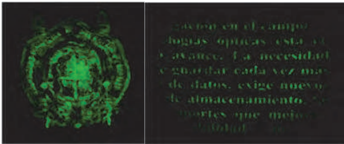
Fig. 24. Real images of the Fourier holograms recorded in our photosensitive material.
