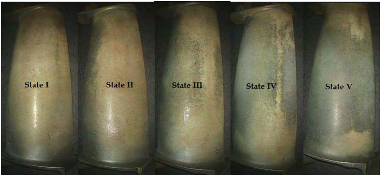
Fig. 17. Recording of vane surface images with a videoscope No. 2
