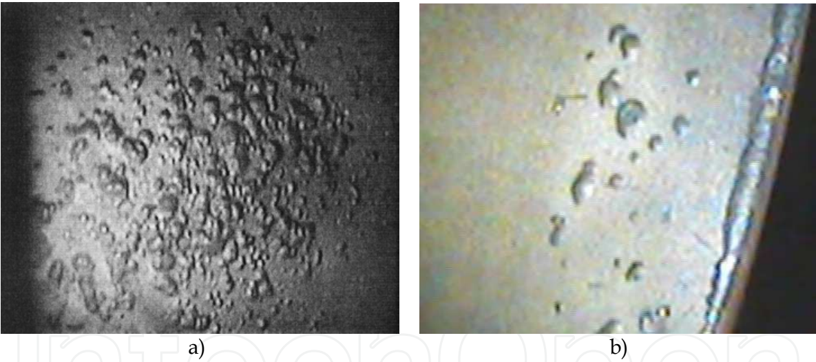
Fig. 9. Failures to turbine blades operated in the seashore environment, caused by chemical impact of exhaust gases (Reports, 2000-2010): a) – on blade surface, b) – on blade leading edge
