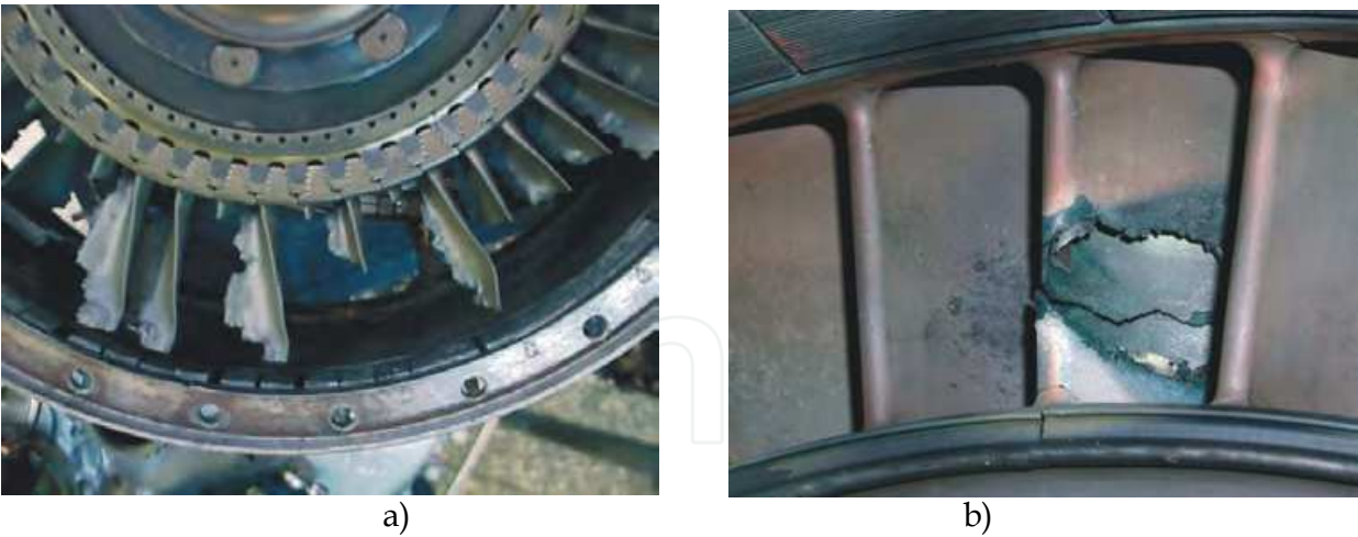
Fig. 8. Characteristic forms of failures to gas turbine caused by long-lasting excessive temperature of exhaust gases (Reports, 2000-2010) : a) – burn-through of turbine rotor blades, b) – melting of a nozzle vane
