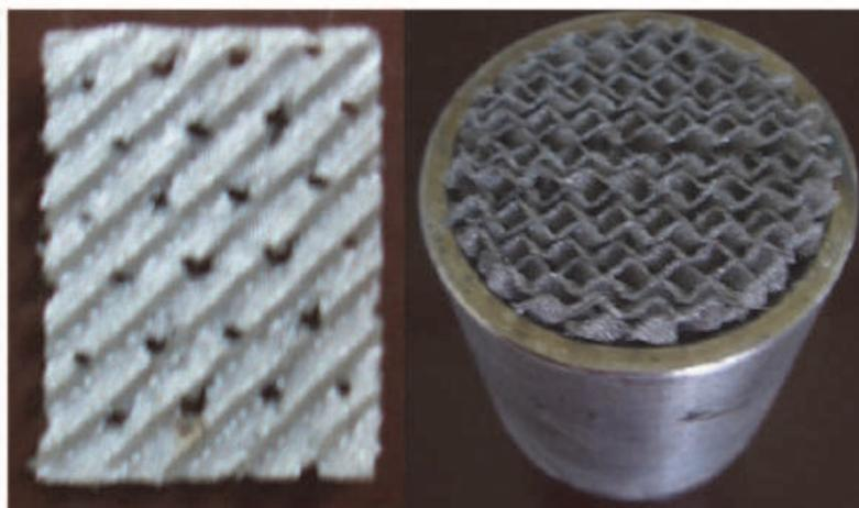
Fig. 6. Illustration of the structured packing PACK-<sup>13</sup>C (Li et al., 2010)
