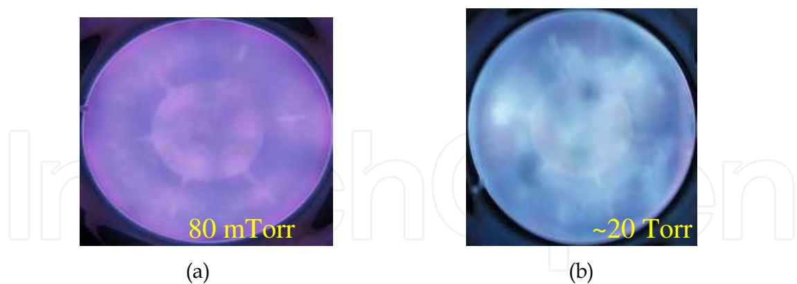
Fig. 4. Images of Ar plasma at a) 80 mTorr and b) 20 Torr. The plasma maintains uniform state under a wide pressure regime.
