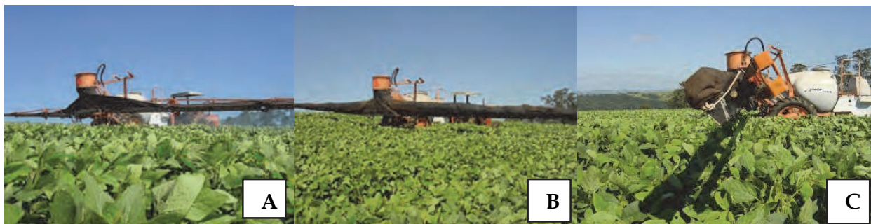
Fig. 3. Air-assisted sleeve boom sprayer in the following operation modes: A – conventional spraying (without air); B – spraying with air assistance at 0° (vertical) and C – spraying with air assistance angled at 30° forward to the displacement of the tractor-sprayer assembly on soybean crop.
