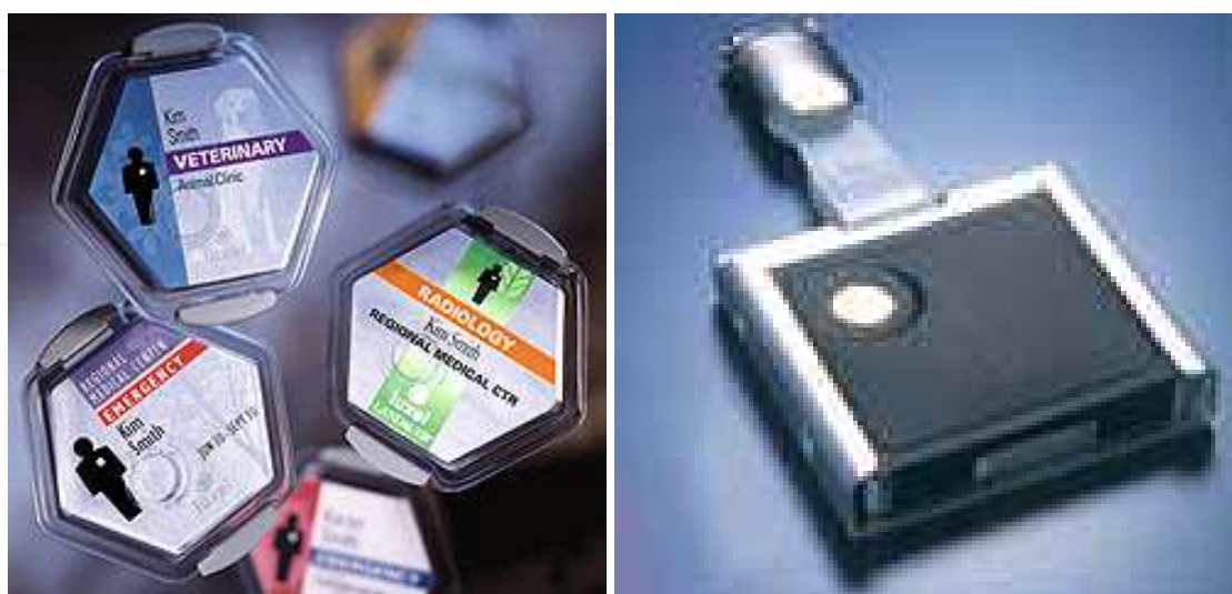
Fig. 7. Photographs of the OSL dosimeter (Type S) as shown the left photo picture and of the DIS dosimetr (Type DIS-1) as shown in the right photo picture.
