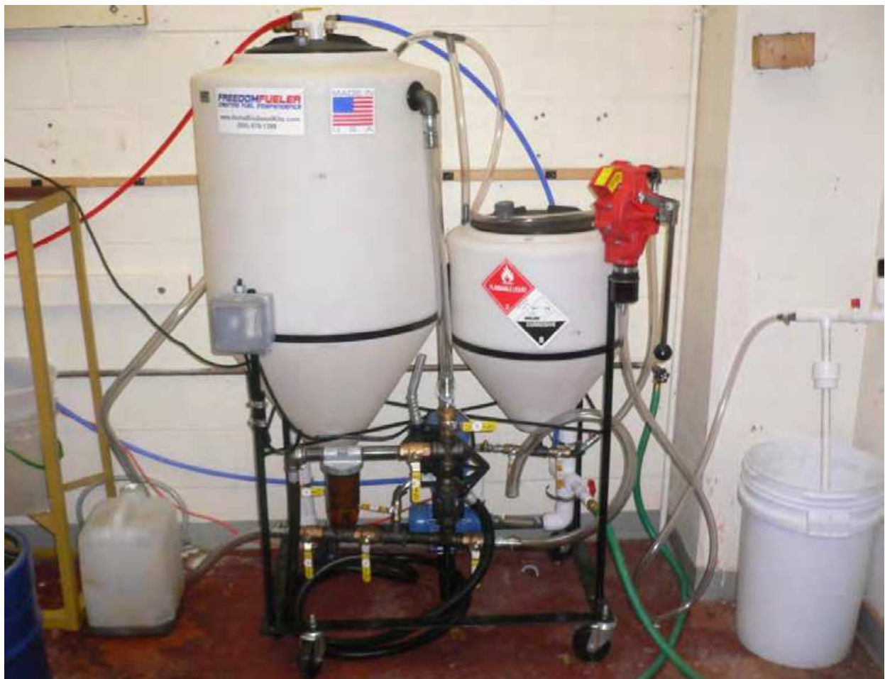
Fig. 3. Biodiesel Processor with a capacity of 40 gallons/day
