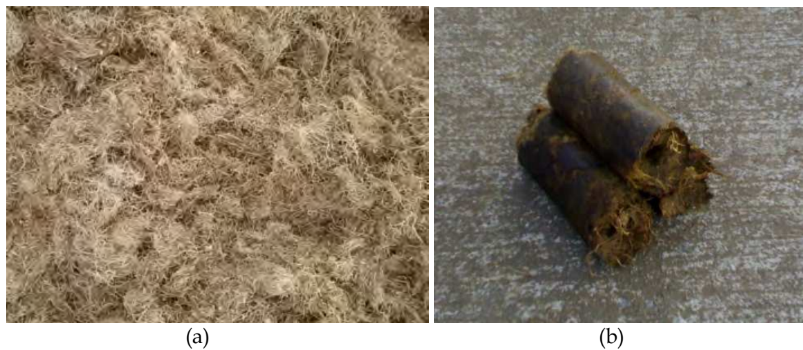
Fig. 9. PEFB before (a) and after (b) pelletizing
