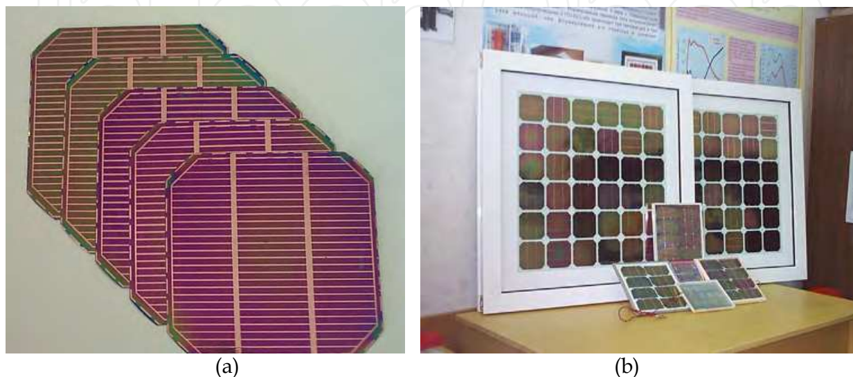
Fig. 22. General view of ITO/nSi photovoltaic converters a) SC with active area 48.6 cm 2 , b) solar modules with different power
