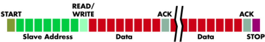
Fig. 16. The I 2 C bus communication
