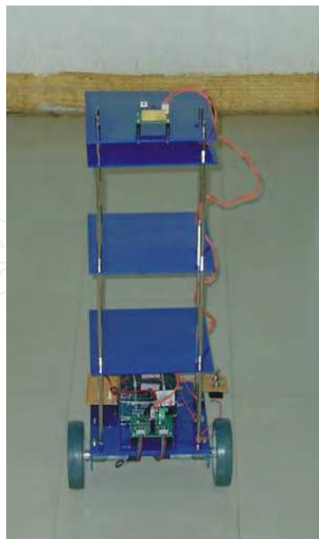
Fig. 17. The Autonomous Mobile Robot (AMRO), Measurement and Mobile robot laboratory
