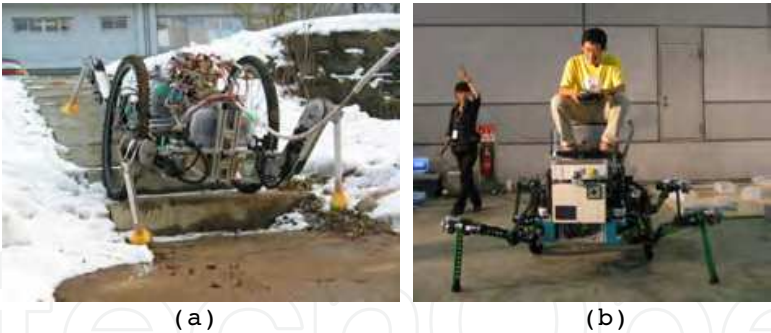
Fig. 1. A leg-wheel robot. (a)Chariot 3. (b)Chari-Bee is a demonstration robot of Aichi EXPO, 2005.
