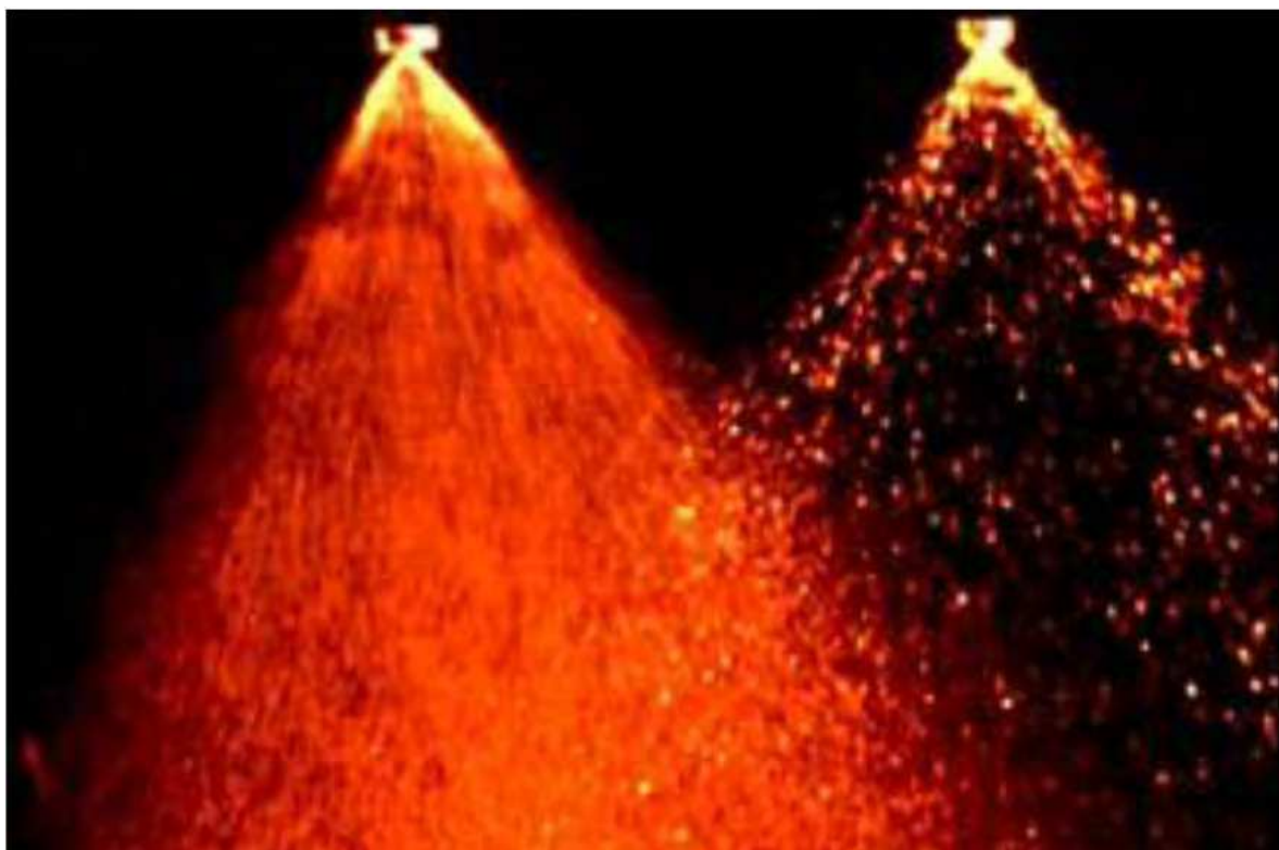
Fig. 1. Effects of nozzle type on the droplet size ( http://www.yorktonaircraft.com/documents/drift.pdf , 2005)
