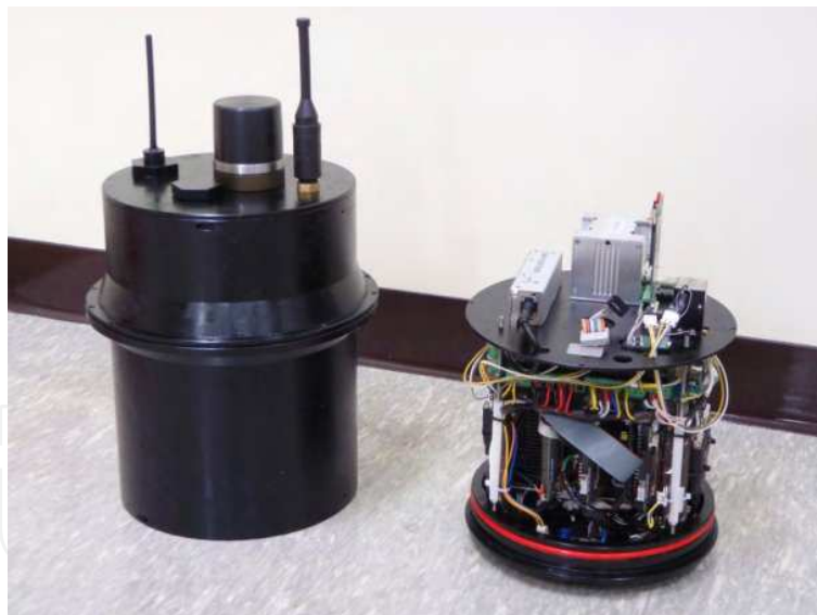
Fig. 3. Electronics system of P-SURO AUV.
