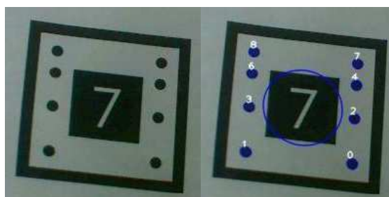
Fig. 5. Designed underwater pattern for P-SURO AUV.
