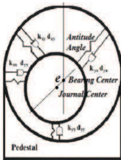
Fig. 17. A linearized model of the hydrodynamic film
