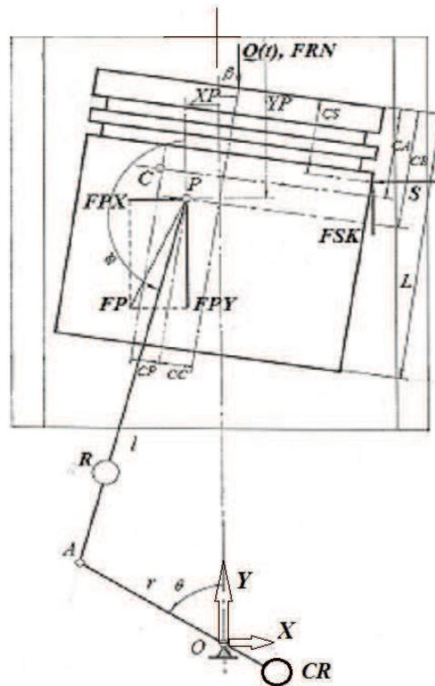
Fig. 6. Cylinder-piston-conrod-crank mechanism
