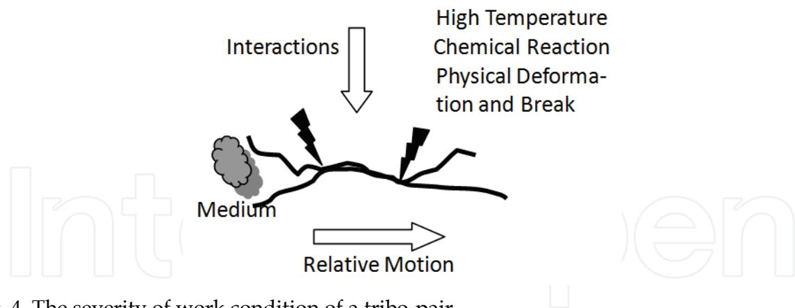
Fig. 4. The severity of work condition of a tribo-pair
