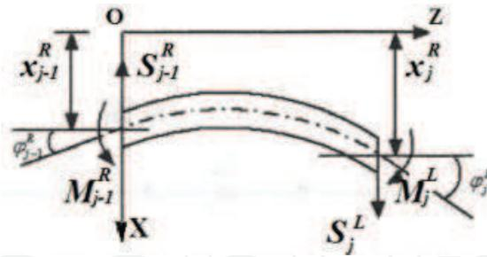
Fig. 15. The lateral deformation of a field
