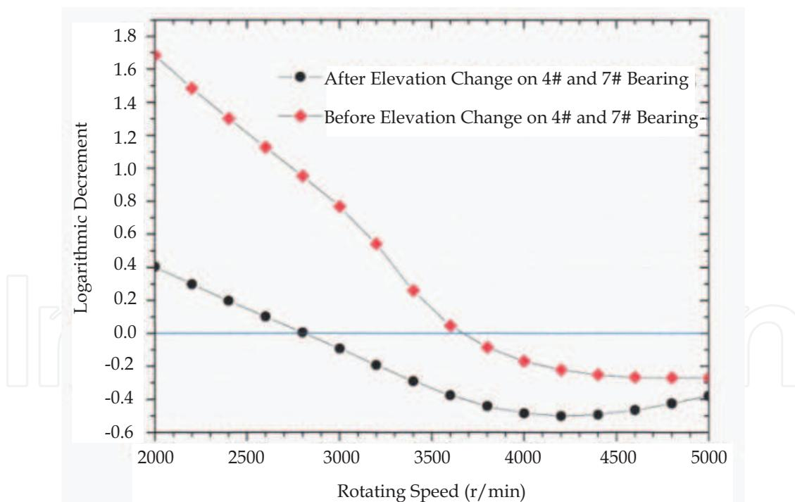
Fig. 18. Logarithmic decrement versus rotating speed for two different elevation distributions
