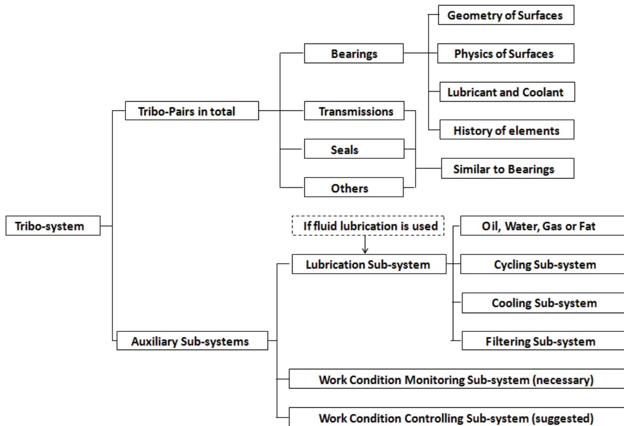
Fig. 2. The block diagram of a typical tribo-system
