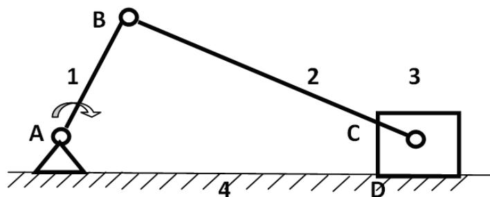
Fig. 1. A crank-slider mechanism
