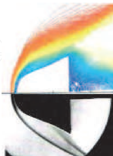
Fig. 4. Comparison between density contour and schlieren picture.
