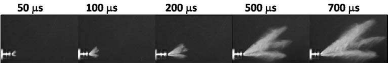
Fig. 5. Sequence of sprays from Injector #2 taken at different time from the SOI at P_{inj} = 10\text{ MPa} , m_f = 50\text{ mg} .
