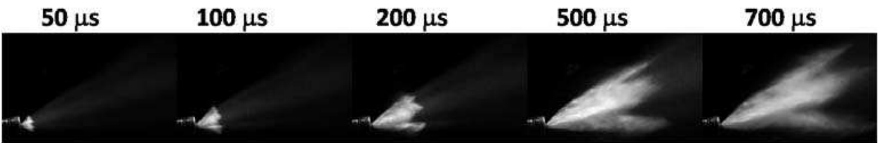
Fig. 4. Sequence of sprays from Injector #1 taken at different time from the SOI at P_{inj} = 10\text{ MPa} , m_f = 50\text{ mg} .
