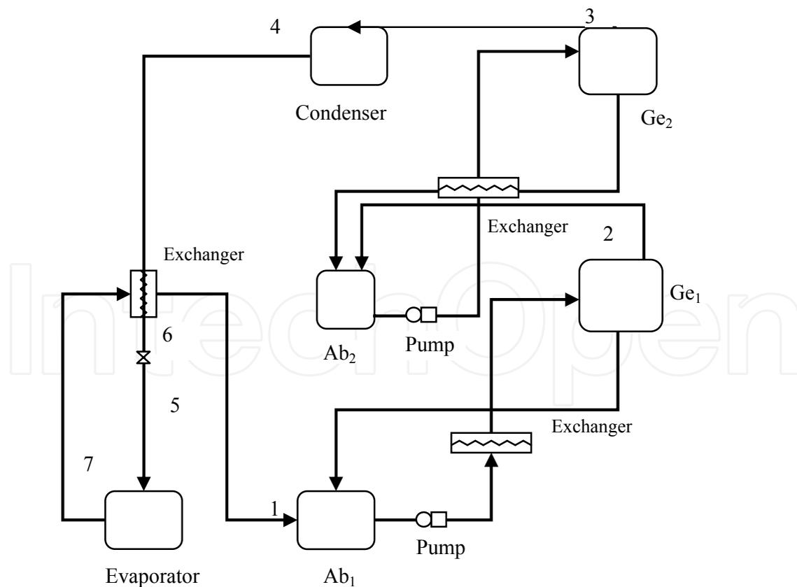
Fig. 4. Absorption machine with double-stage
