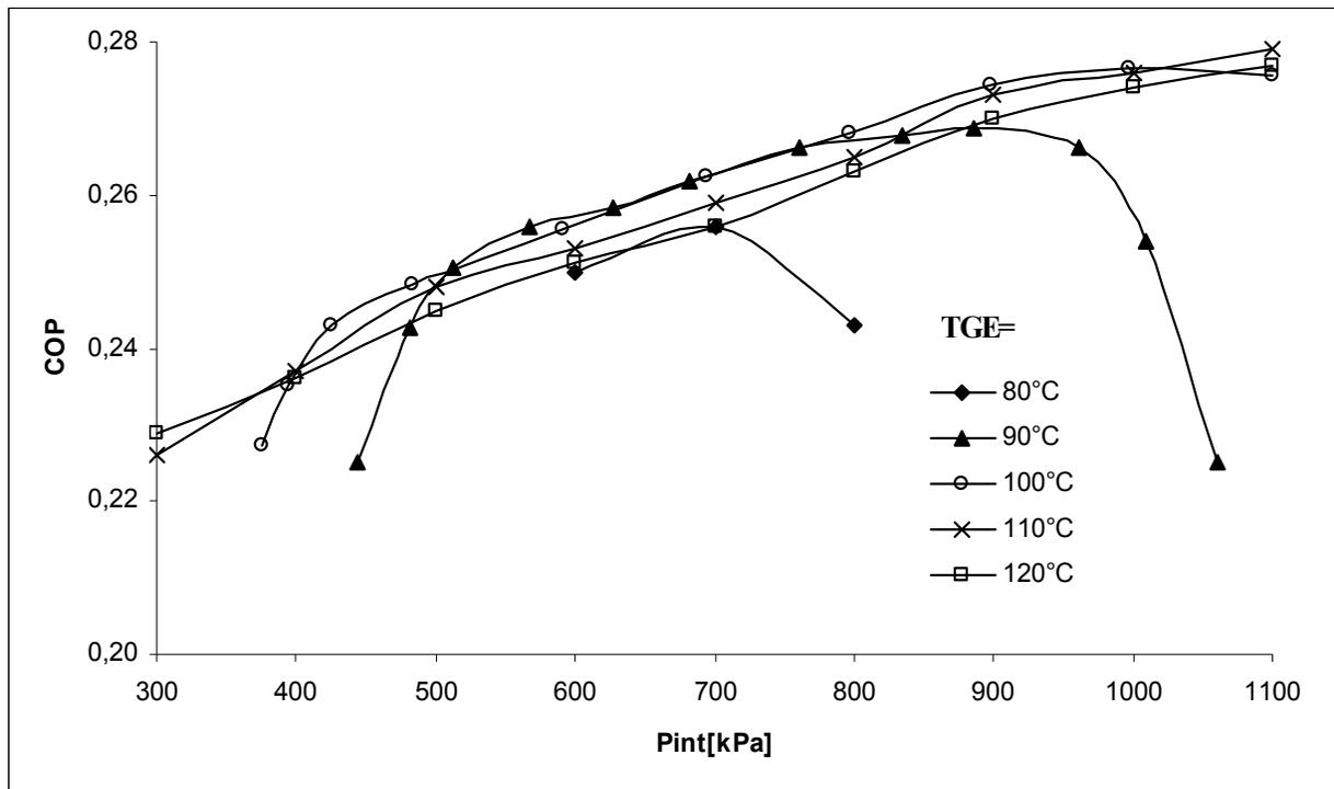
Fig. 20. COP evolution versus P<sub>int</sub> with T<sub>CD</sub>=40 C and T<sub>EV</sub>= -10 C
