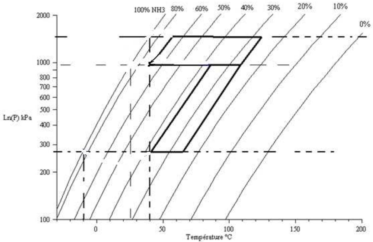
Fig. 6. Oldham Diagram of system AGEcAG
