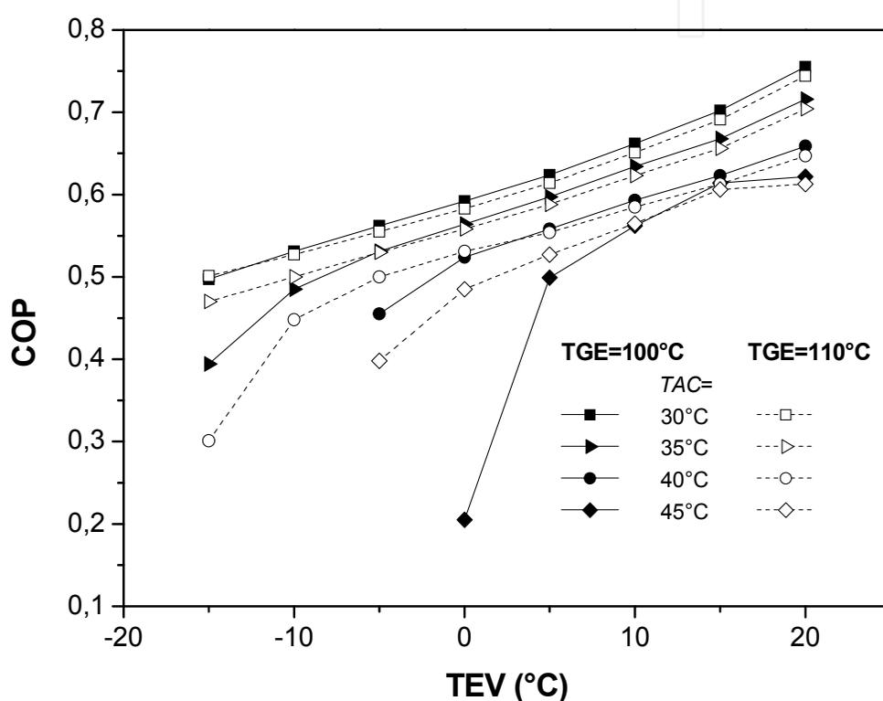
Fig. 13. COP evolution versus  $T_{EV}$  for different  $T_{AC}$  temperature and  $T_{GE} = 100$  C and 110 C
