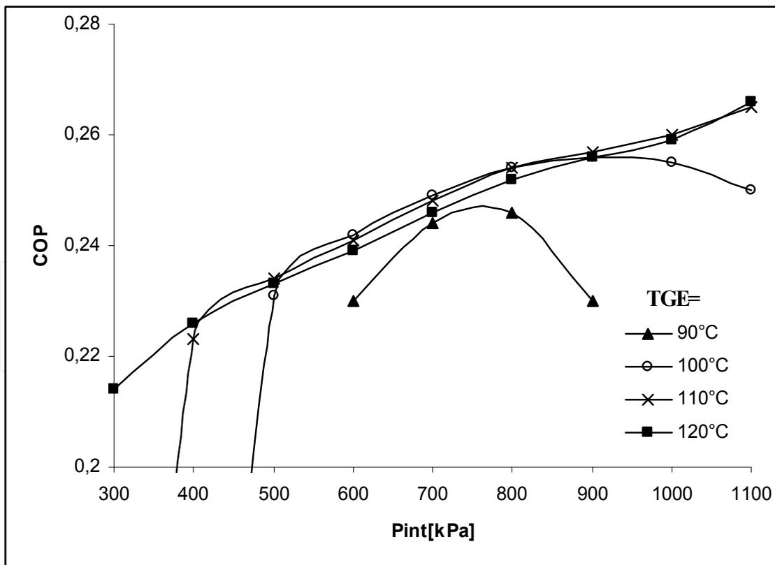
Fig. 21. COP evolution versus P<sub>int</sub> with T<sub>CD</sub>=45 C and T<sub>EV</sub>= -10 C
