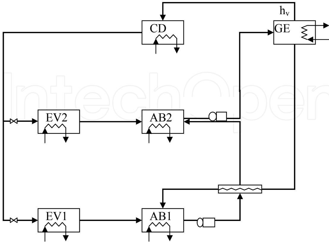
Fig. 9. System AAG (connection absorber-absorber)
