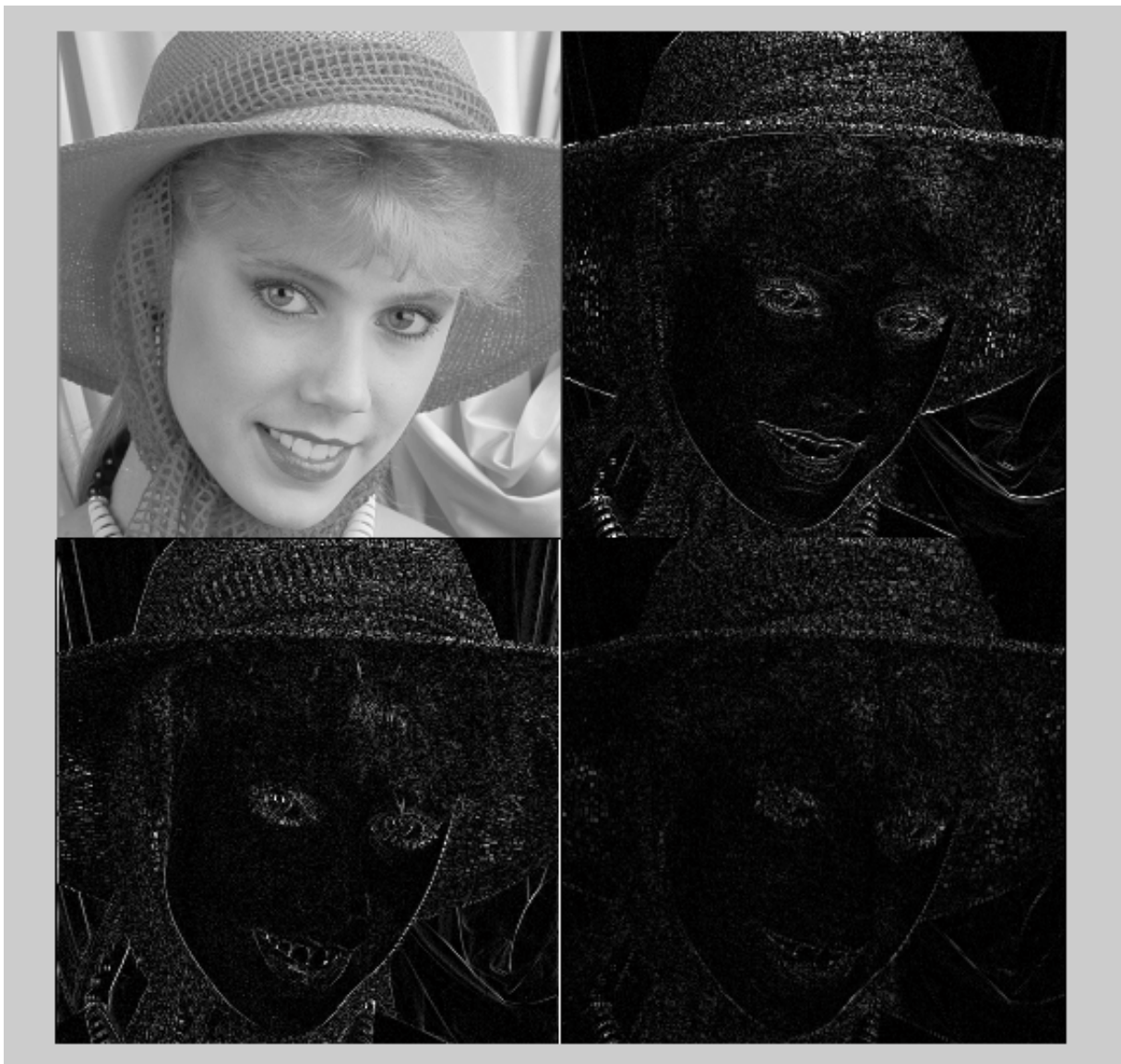
Fig. 12. Single level wavelet decomposition
