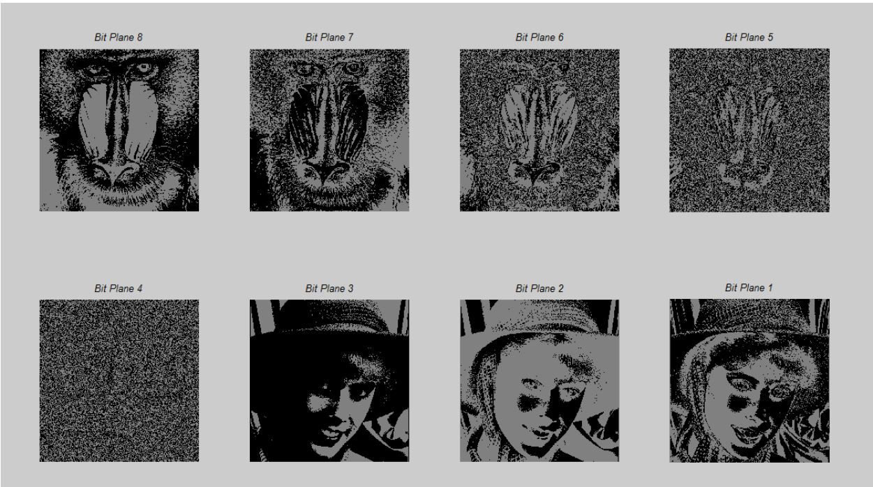
Fig. 4. Substituting the LSB(s) of the asset with MSB(s) of the message
