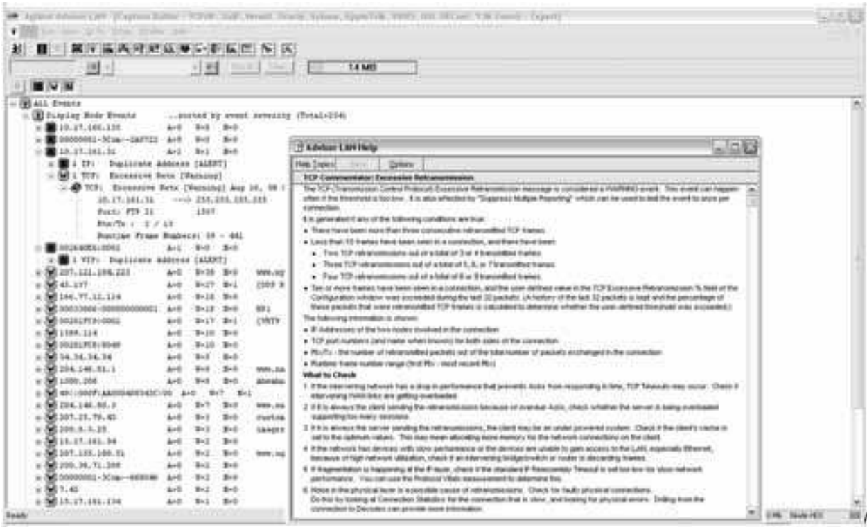
Fig. 10. An example of expert analysis based detection, isolation and classification of excessive TCP transmissions
