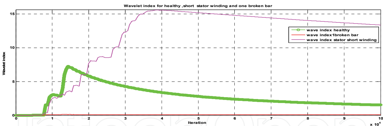
Fig. 14. Wavelet index for fault detection
